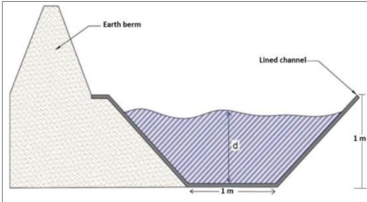
**Figure 5-1: Typical drain adjoined to a berm for stormwater channelization**
