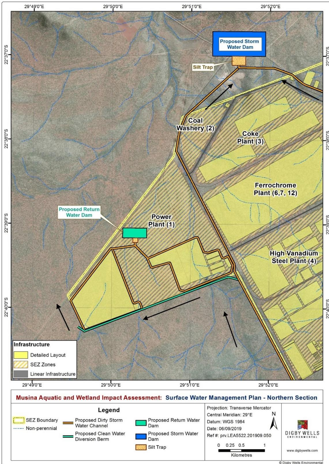
**Figure 5-4: Proposed Storm Water Management Plan**
