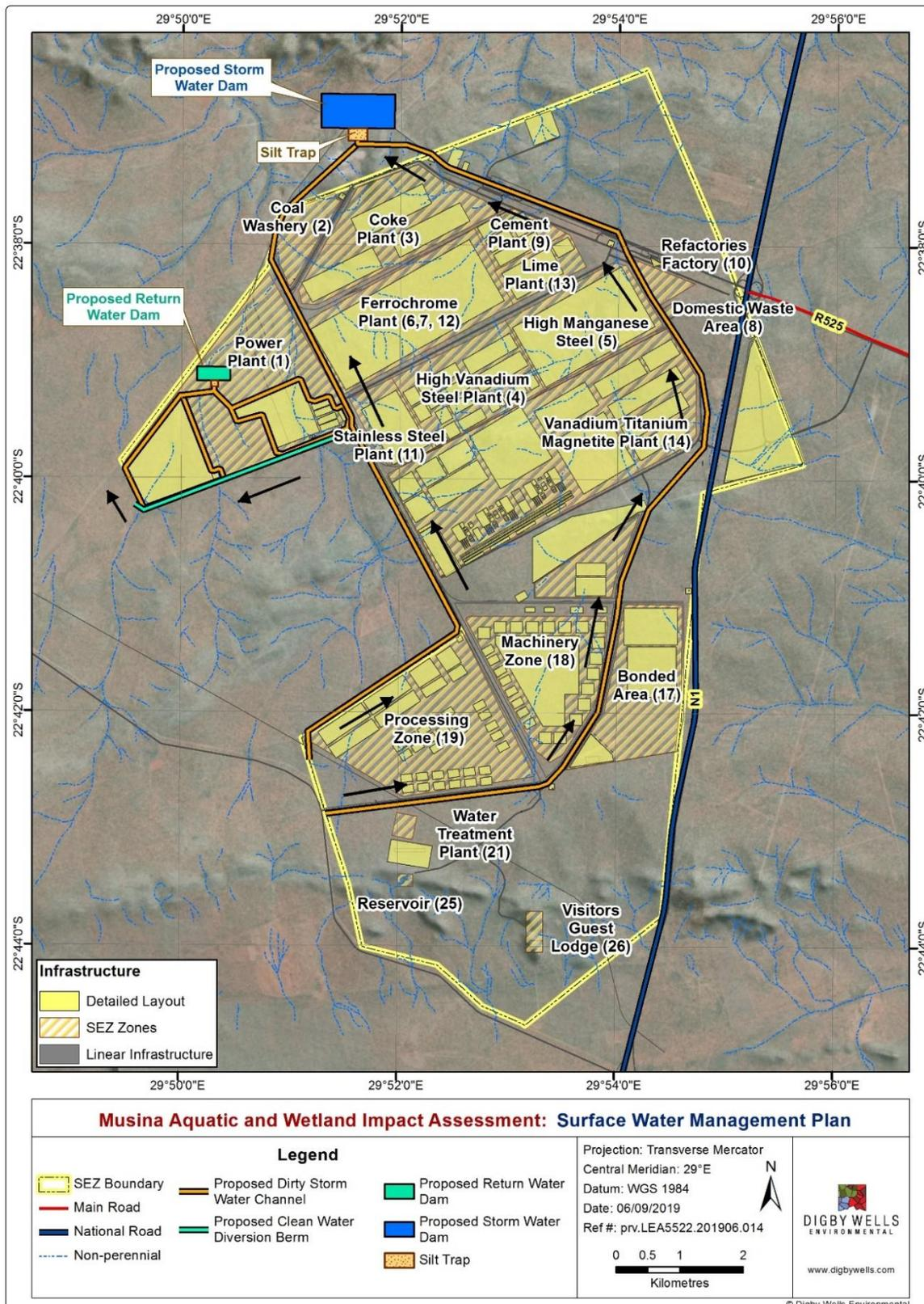
**Figure 5-3: Proposed Storm Water Management Plan**
